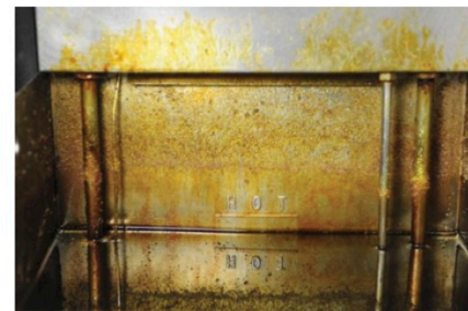
Fryers were used to prepare French fries over 13 days at 176° C, 8 hours per day.
