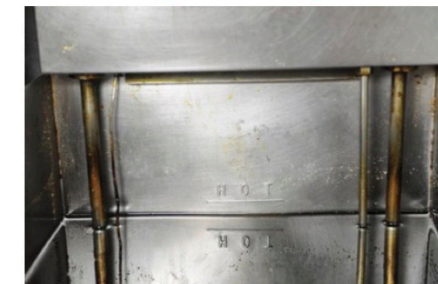
Fryers were used to prepare French fries over 13 days at 176° C, 8 hours per day.
